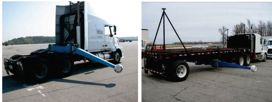
AP Figure 1. Tractor and trailer mounted outriggers.
