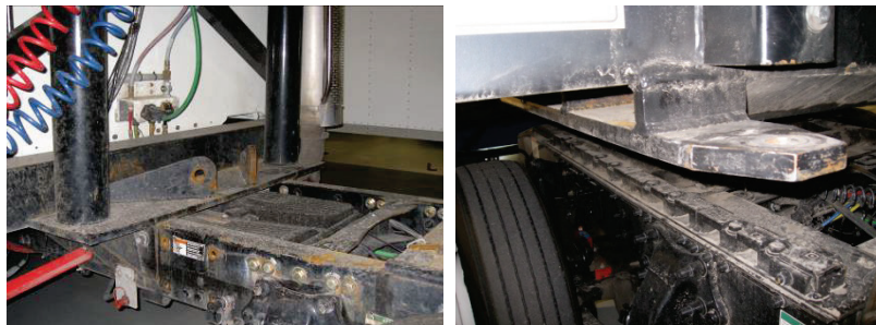
AP Figure 2. Anti-jackknife mounts on tractor and trailer.
