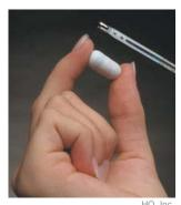
The CorTemp pill, from HQ Inc., has a built-in battery and wirelessly transmits real-time body temperature.
