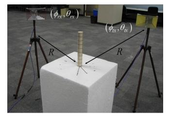
**Figure 7.** Far-field bistatic measurement setup. As shown in the schematic, the transmitter ( $\phi_{tx}$ ,  $\theta_{tx}$ ) and the receiver ( $\phi_{rx}$ ,  $\theta_{rx}$ ) are both at distance  $R = 17.5\lambda_0$  from the region under test.
