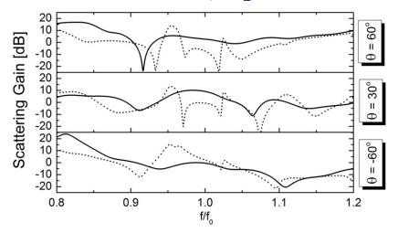
**Figure 11.** Bi-static scattering gain for  $\phi_{tx,rx} = 0^{\circ}$  and various elevation angles: measurements (solid) and simulations (dotted) are compared in each panel.
