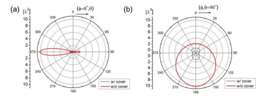
**Figure 6.** Principal plane elevation (a), and azimuthal (c) scattering profiles at 3.73 GHz.
