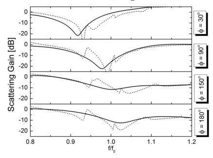
**Figure 10.** Bi-static scattering gain for normal incidence  $30^{\circ} \le \phi \le 180^{\circ}$ ,  $\theta_{rx,tx} = 90^{\circ}$  and various azimuthal receiver angles: measurements (solid) and simulations (dotted) are compared in each panel.
