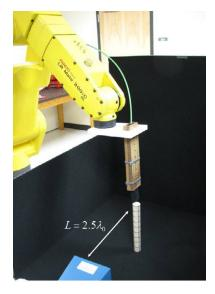
**Figure 8.** Picture of the near-field mapping system. A microwave horn excites each test scenario and a near-field probe samples the temporal and spatial TM-polarized electric field.
