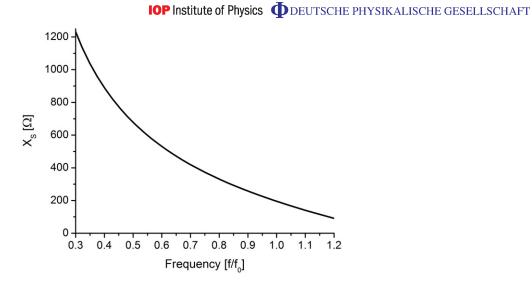
**Figure 2.** Required surface reactance to suppress the dominant scattering order for the geometry of figure 1 illuminated by a TM-polarized plane wave at normal incidence.
