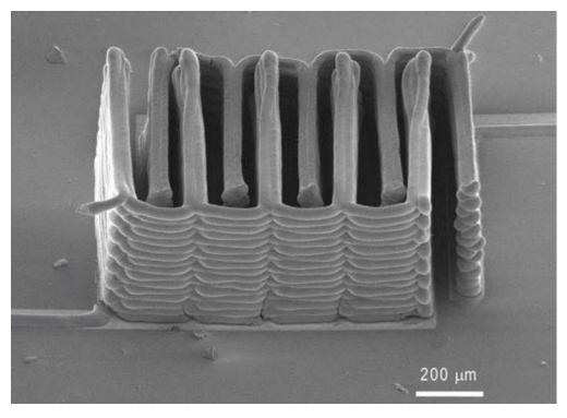
A research team from Harvard University and the University of Illinois at Urbana-Champaign has demonstrated the ability to 3D print a battery. This image shows the interlaced stack of electrodes that were printed layer by layer to create the working anode and cathode of a microbattery. (SEM image courtesy of Jennifer A. Lewis.)
