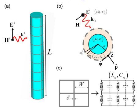
**Figure 1.** Magnetodielectric cylinder covered by a mantle metascreen and excited by a TM-polarized plane wave at normal incidence (a). Cross-section of the cylinder and of the conformal metascreen (b). Inductive surface reactance realized by a *fishnet* metascreen composed of subwavelength frequency-selective surface elements and its lumped equivalent circuit (c).
