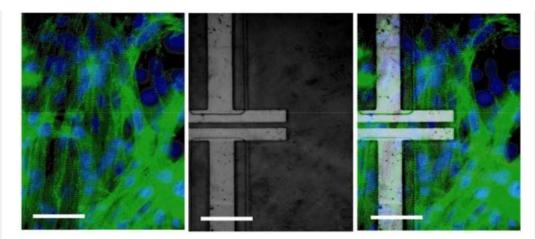
Cardiac cells, with a nanoelectroic electrode highlighted
