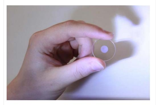
To read these spots, an optical microscope that's capable of untangling the polarized light reflected by the three-bit spots is used. There's no word on whether these silica glass discs can be rewritten, but the research paper [PDF] makes it sound like this is a write-once-read-many (WORM) storage method.
