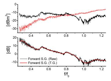
**Figure 9.** (a) Raw RCS data measured in the forward direction of the uncovered (dashed) and covered (solid) cylinder; (b) comparison of the computed scattering gain (S.G.) in the same direction obtained from raw RCS data and time-gated (T.G.) data.
