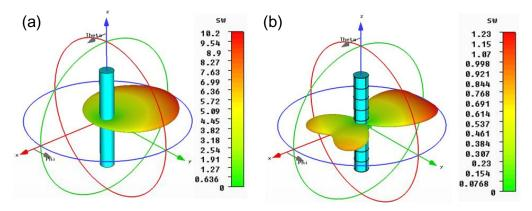
**Figure 5.** 3D far-field total scattering profiles for the uncloaked (a) and cloaked cases (b) at 3.73 GHz.
