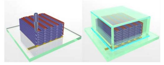
To create the microbattery, a custom-built 3D printer extrudes special inks through a nozzle narrower than a human hair. Those inks solidify to create the battery's anode (red) and cathode (purple), layer by layer. A case (green) then encloses the electrodes and the electrolyte solution is added to create a working microbattery. (Illustration courtesy of Jennifer A. Lewis.)
